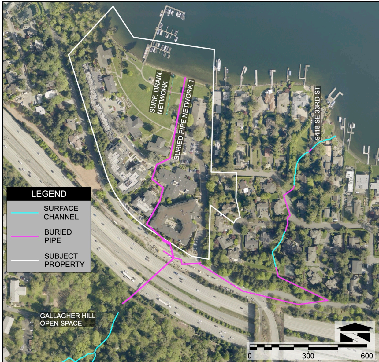
Figure 7 - Buried Pipe Network 1 and Historic Route
